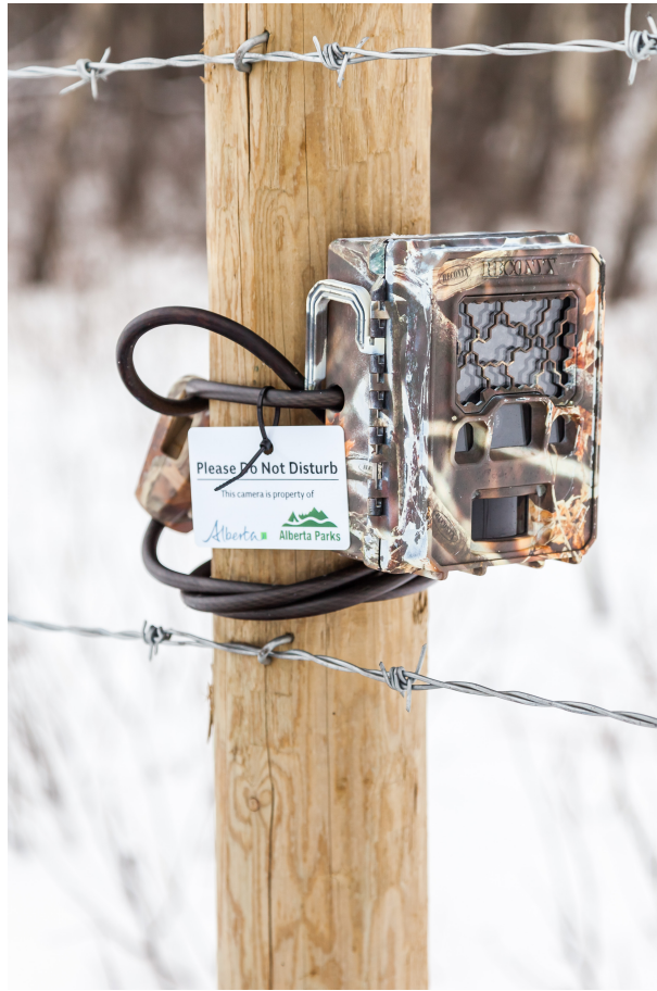
Figure 2: Reconyx camera and placement on the fence, in this case a wildlife friendly fence. Photo courtesy of Drajs Vujnovic.
