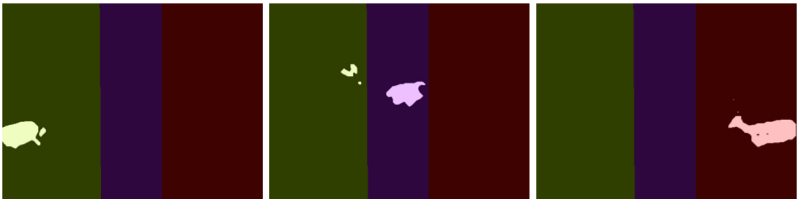
Figure A.9: The example crossing sequence difference images following thresholding, erosions and dilation.
