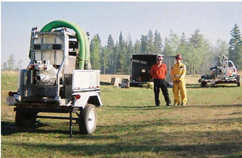
*Figure 9.3. Portable pump (Rapid Fire and Rescue Inc.).*
