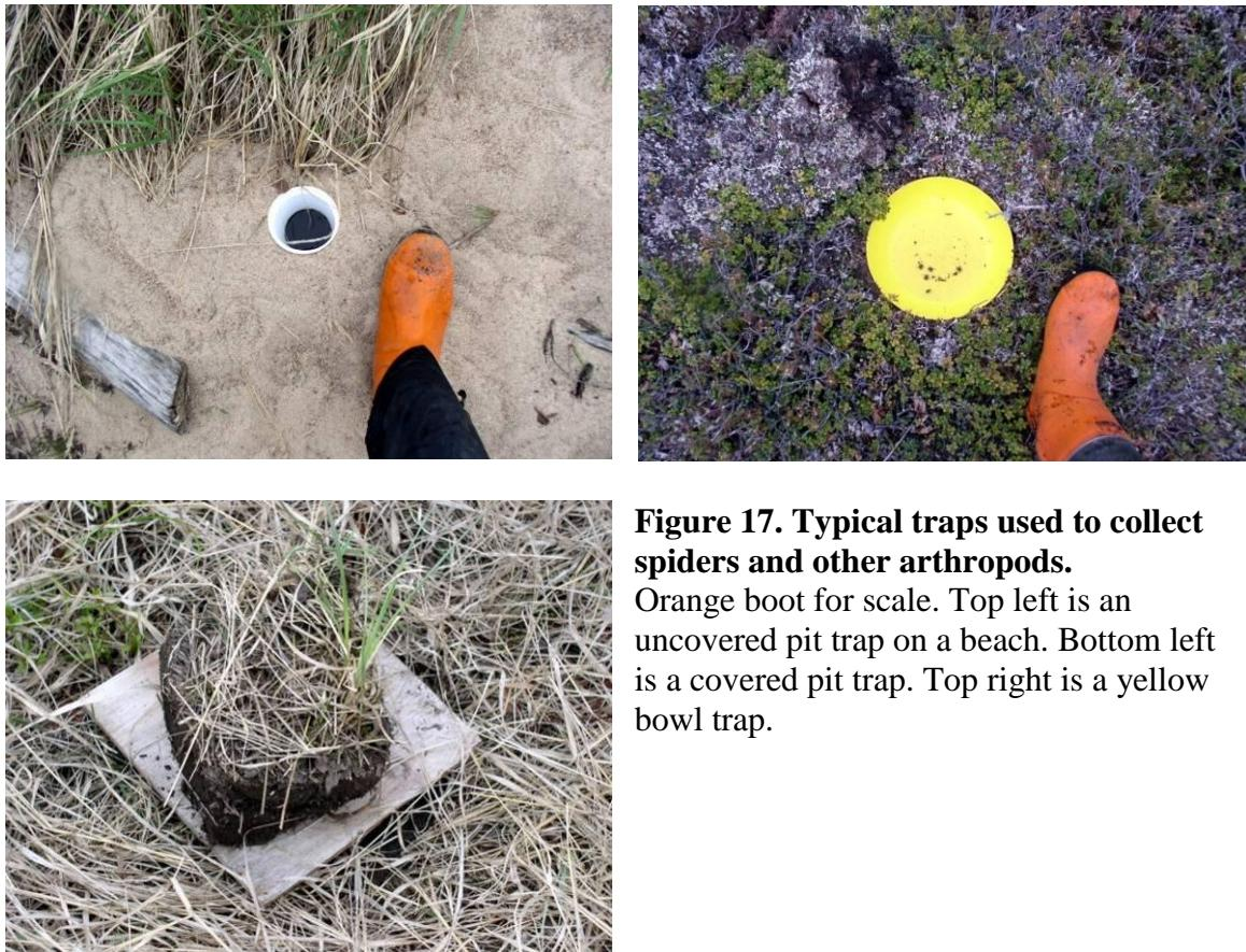
**Figure 17. Typical traps used to collect spiders and other arthropods.**
