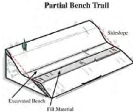
On a partial bench trail, only part of the hill is cut away and the soil that has been removed is placed at the lower edge of the trail to try to establish the desired tread width.
